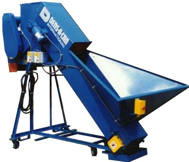
**DENS-A-CAN Portable Glass Breaker with optional remote stop**
